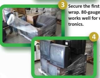
Secure the first layer with strech wrap. 80-gauge strechwrap works well for wrapping electronics.
